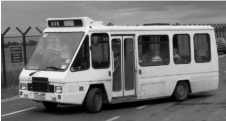
Figure 2. Innovative CVE ‘Omni’ low-floor bus, c.1994. (source: http://www.irishbuses.com , 2012, © Darren Hall)
